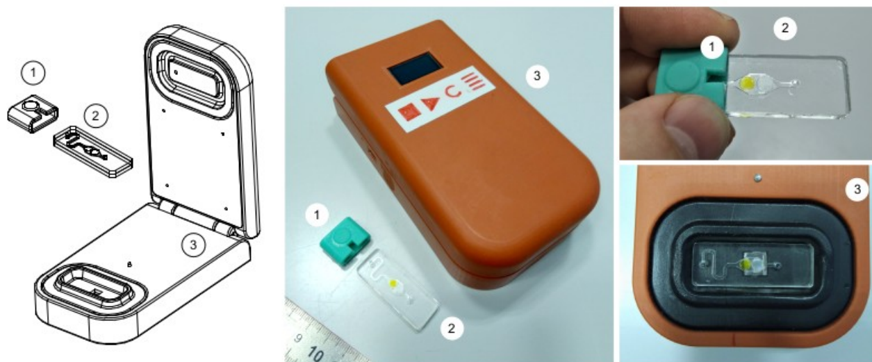
Figure 1. The biosensor consists of a SiPM-based handheld luminometer (3), a disposable microfluidic chip (2) and a sampler adapter for chips (1). The portable luminometer has the capability of autonomous operation, for this purpose it is equipped with a battery, a display and control buttons. The disposable microfluidic chips contain enzymes and substrates of the coupled enzyme bioluminescent system NAD(P)H:FMN-oxidoreductase+luciferase co-immobilized into starch gel.
